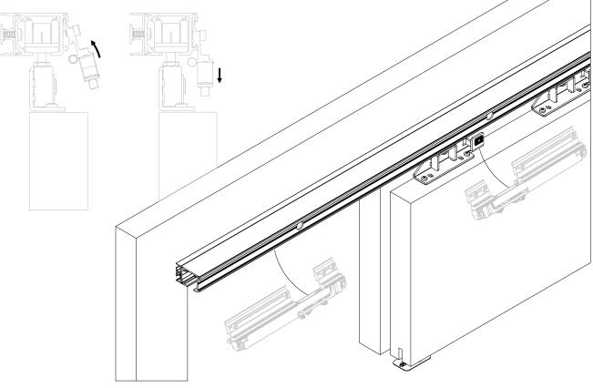
**Step 6**Fixing the activator to the wood holder
