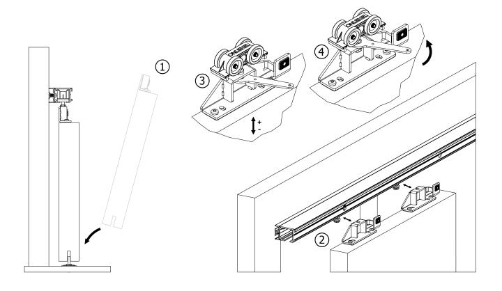
**Step 5**Swivelling the dampers into the guide rail
