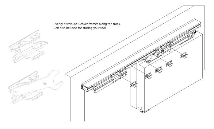
**Step 9**Mounting the cover profile to the running track
