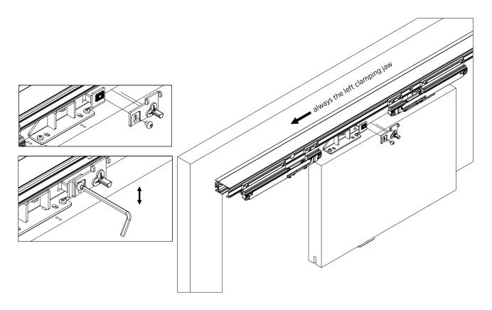
Step 7 Sliding the activator into the damper
