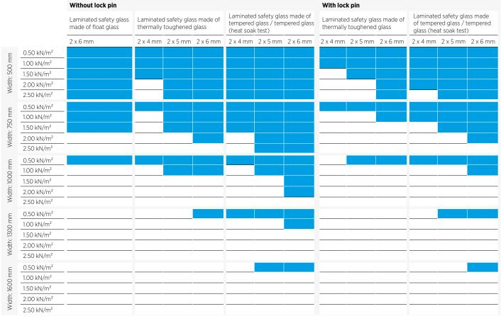
complies with DIN 18008 does not comply with DIN 18008
